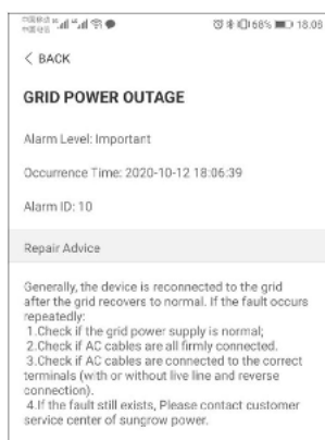
Figure 7-10 Detailed Fault Alarm Information
