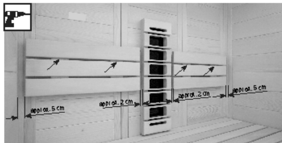
3 mm drill bit, 4 screws 4 x 70 mm
